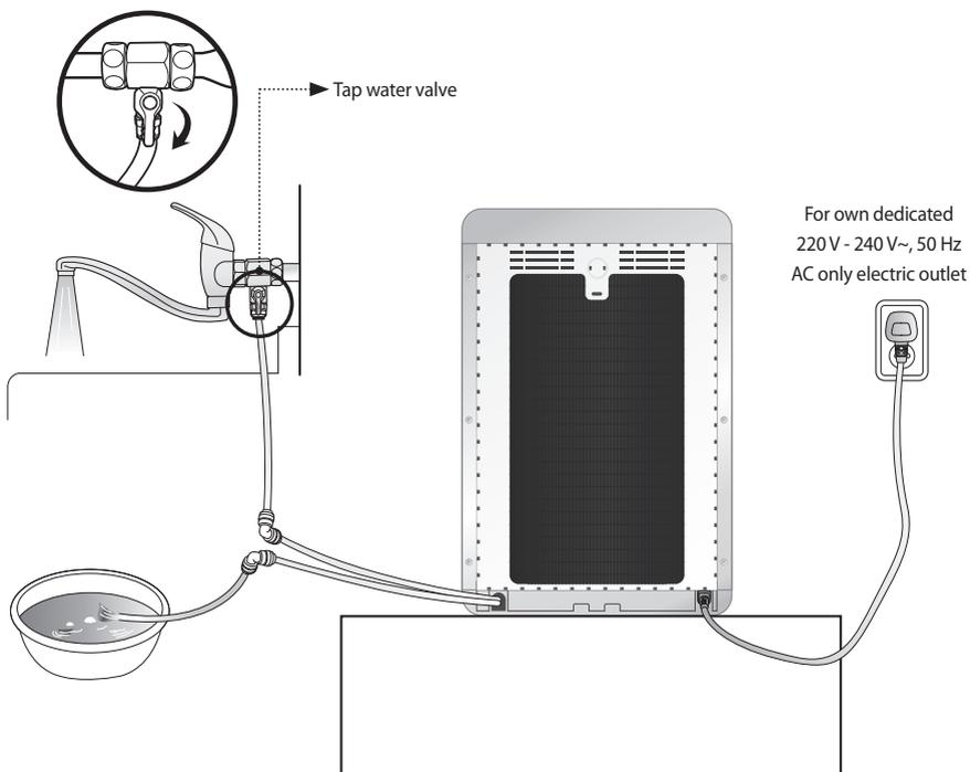
Connect the orange tap water input hose to **1** the water pipe.
