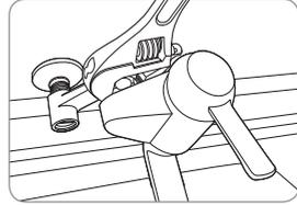
2. Wind the teflon tape on the adaptor and fit it to the pipe.
