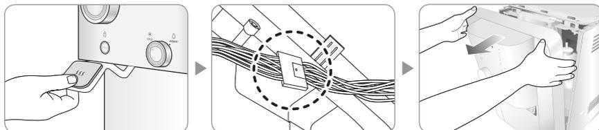
5. After separating the fitting connected to the filter, please replace the filter.
