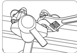
4. Connect ¼ inch orange tubing with the connector on the adaptor.
