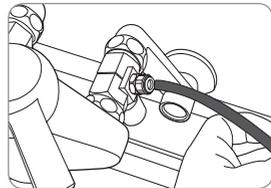
5. Connect it to a socket with voltage rating that matches the one stated on the rating plate. Then, open the feed valve to supply water to the filtration system.
