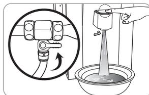
2. Open the side draining door and pull out the red draining faucet. Empty the water tank completely using the draining hose and unplug the power cord.
