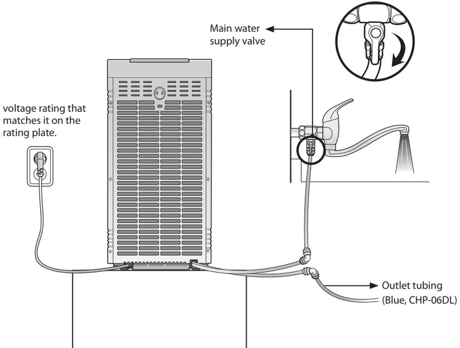
Connect the orange color inlet tubing ① to the tap water supplying pipe. Connect the outlet tubing(CHP-06DL) ②.
