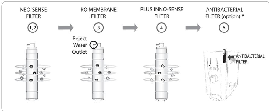
\* The Antibacterial filter contains silver, which is known to inhibit the propagation of microorganisms and to maintain the integrity of the filter.
