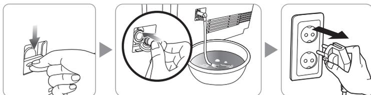
3. Please remove the top cover, and then un-hook the fixed clip holding the top cover of the water tank. Now remove hose and open the tank cover.
