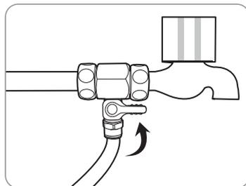
2. After separating the fitting connected to the filter to replace, please replace the filter. (Separate the fitting using the proper tool.)
