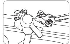
4. Connect 1/4 inch orange tubing with the connector on the adaptor.
