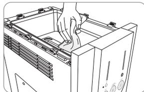
6. Use the storage tank after cleaning it with the drained water, plug-in the power cord, then empty the water tank using the draining hose and continuous extraction method. After cleaning, please close both tank and top cover, then empty the water tank filled with filtered water one more time.
