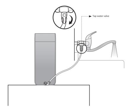
Connect the orange tubing to (1), and the tap water pipe.
