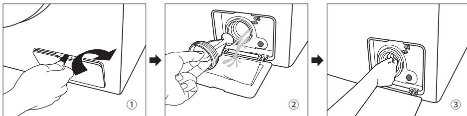
Open the filter cover with tools such as coins according to the direction of the graphic;
